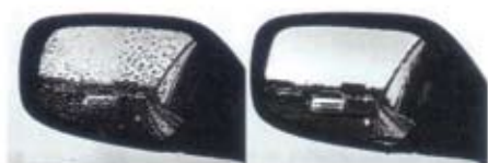
Fig. 19: Anti-fogging effect of automobile side-view mirror: conventional mirror (left) and TiO 2 -coated mirror (right).
