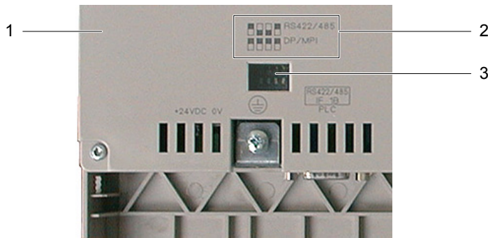
Figure 4-12 Position of the DIL switch on the OP 170B
